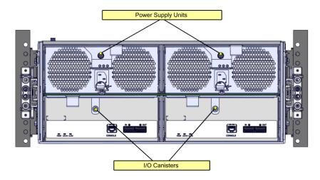
Figure 4: Identification of Assembled Enclosure (Hard Drive Assembly)
