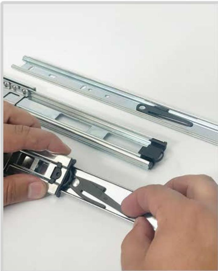
**REMOVE INNER MEMBER** by depressing the release latch, pictured at left, and sliding the inner member completely out of the slide assembly as pictured at top.
