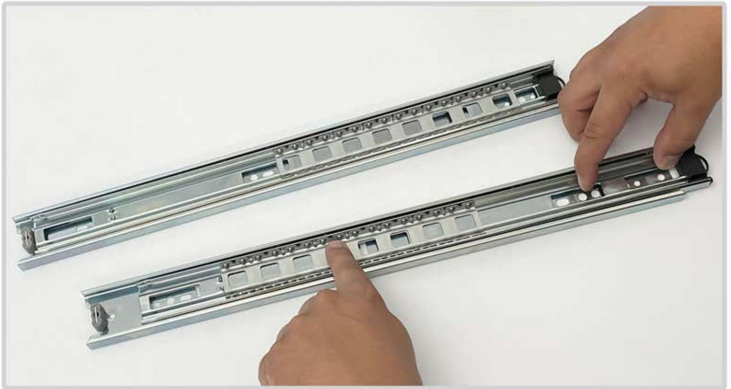
The first step is to roll the inner ball bearing retainer bracket to the rear of the intermediary slide bracket. Picture above shows the ball bearing retainer in normal position, and the slide to the rear.
