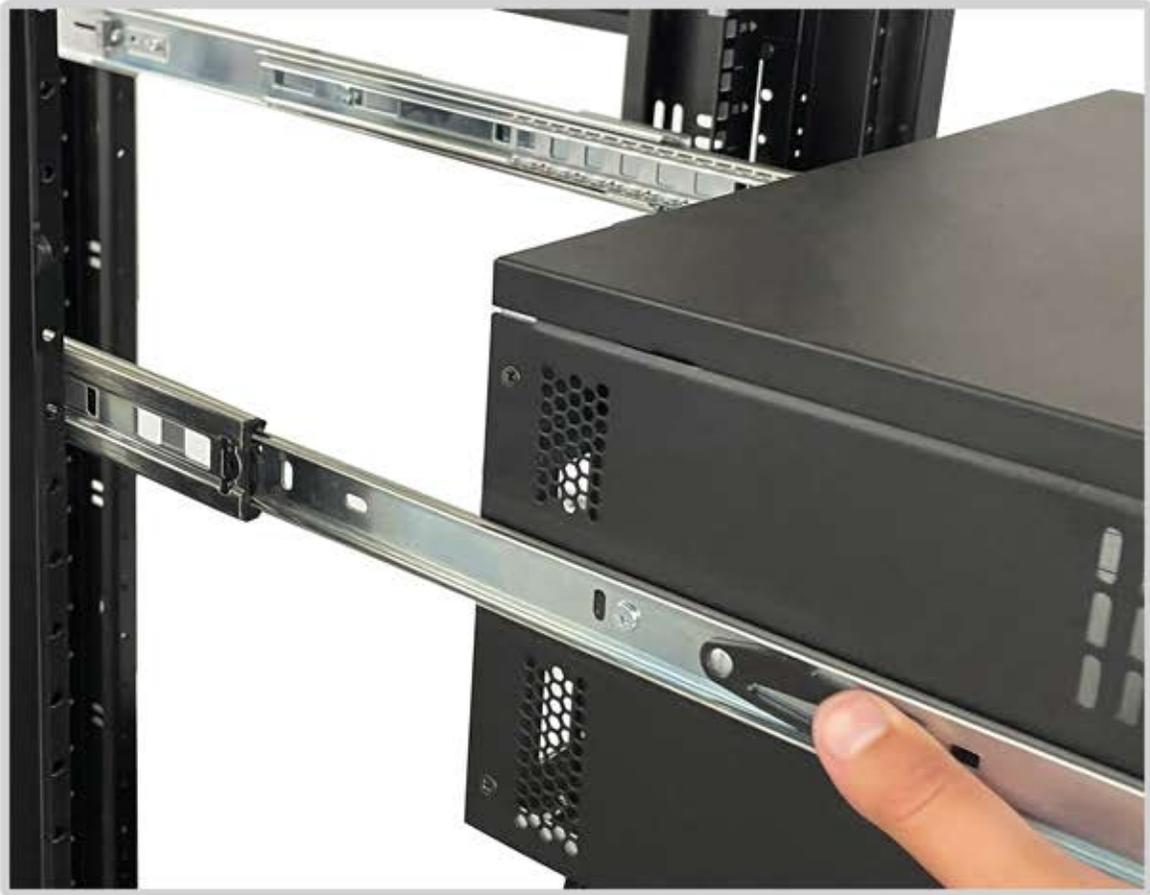
Once both rack slide assemblies are successfully installed into your rack cabinet, it is time to slide your CX rack chassis into position.
