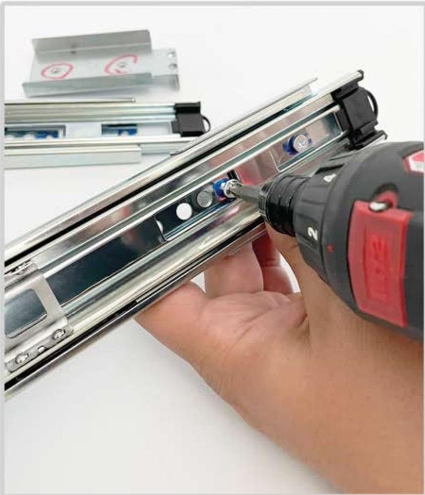
Note that you will need to slide the middle member of the rail assembly out a little bit to get access to the required holes.
