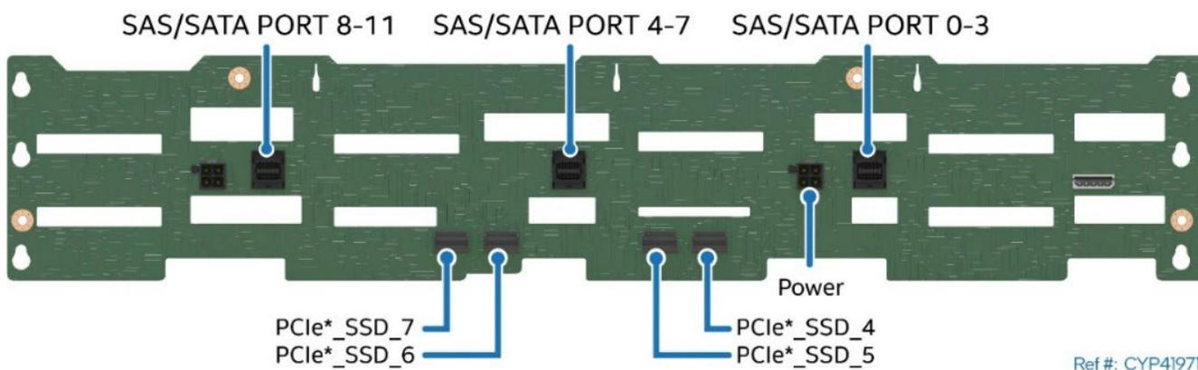
**Figure 79. 12 x 3.5" HSBP Connector Identification – Back Side**
