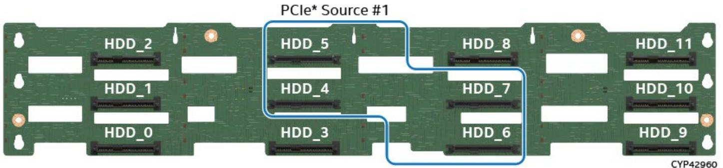
**Figure 86. 12 x 3.5" HSBP NVMe\* Connector Identification – Front Side**
