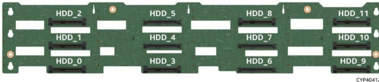
**Figure 78. 12 x 3.5" HSBP Connector Identification – Front Side**
