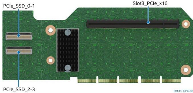
**Figure 49. PCIe\* NVMe\* Riser Card for Riser Slot #1**
