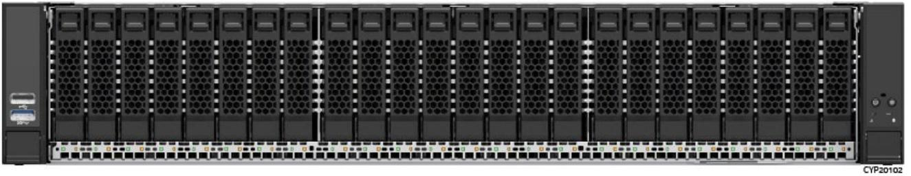
**Figure 10. 24 x 2.5" Front Drive Bay Configuration (M50FCP2UR208 with optional accessories)**
