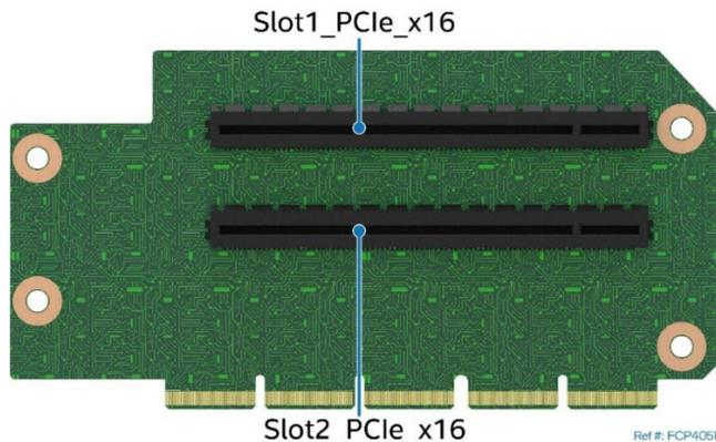
Figure 48. Two-Slot PCIe\* Riser Card for Riser Slot #1
