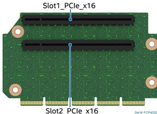
**Figure 52. Two-slot PCIe\* Riser Card for Riser Slot #2**
