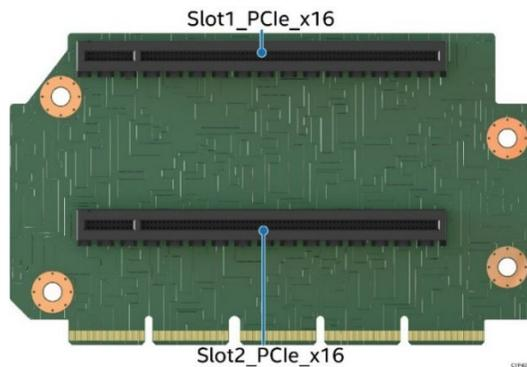
**Figure 51. Two-slot PCIe\* Riser Card for Riser Slot #2**
