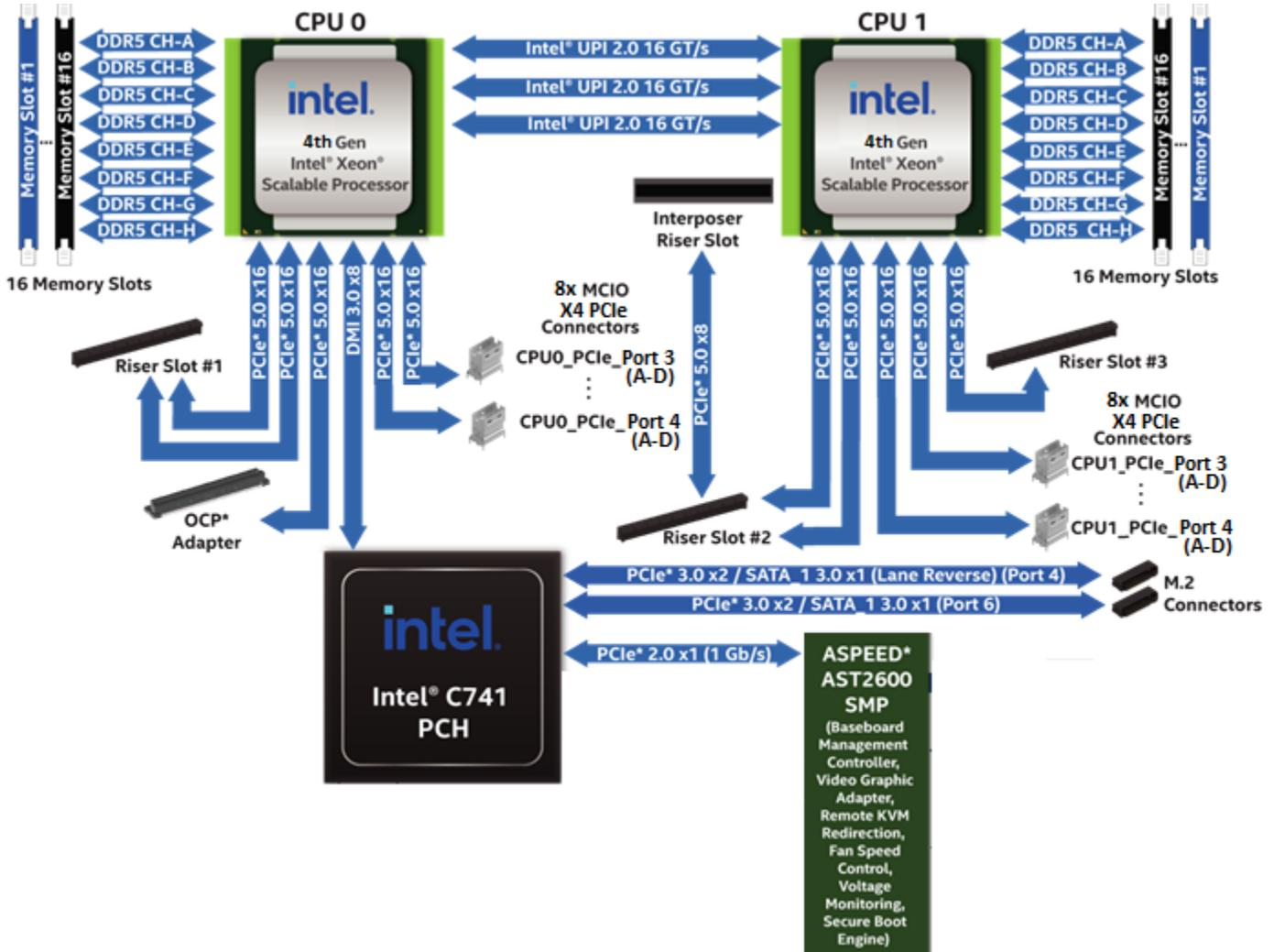
Figure 40. PCIe Subsystem Architecture
