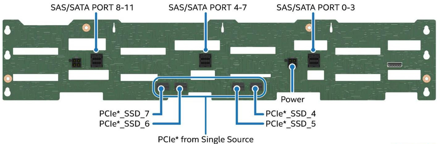
**Figure 87. 12 x 3.5" HSBP Connector Identification – Back Side**
