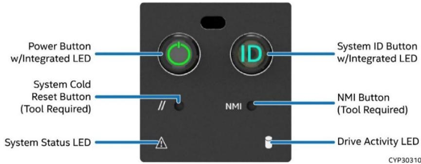
**Figure 93. Front Control Panel Features**
