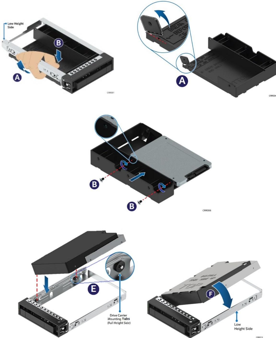
**Figure 66. 2.5" SSD Assembly into Drive Rail – Alignment and SSD Installation**
