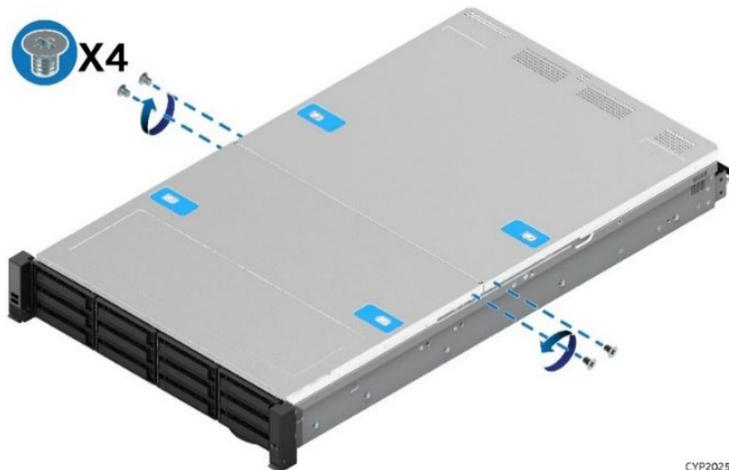
**Figure 23. Top System Cover Panels Shipping Screws**
