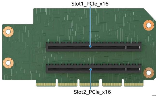
Figure 47. Two-Slot PCIe\* Riser Card for Riser Slot #1
