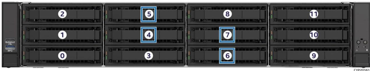
**Figure 77. 12 x 3.5" Front Bay Drive Configuration – M50FCP2UR312**
