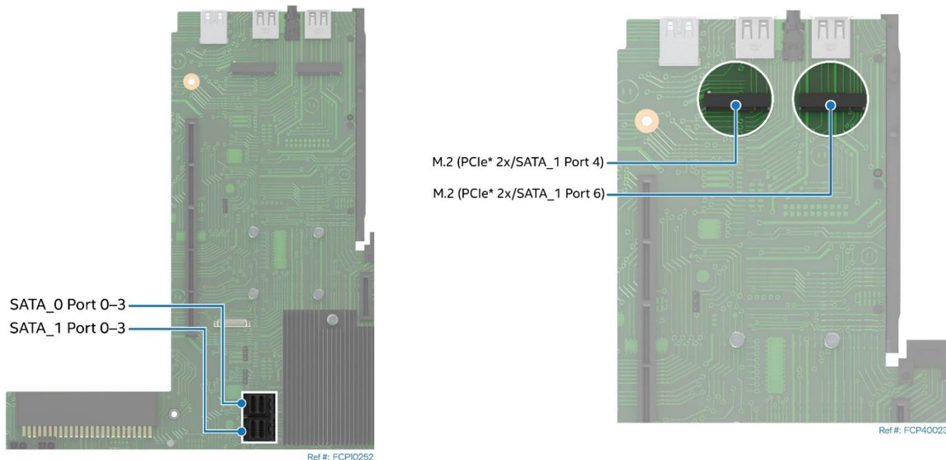
**Figure 88. Onboard SATA Cable Connectors and M.2 SSD Connectors**
