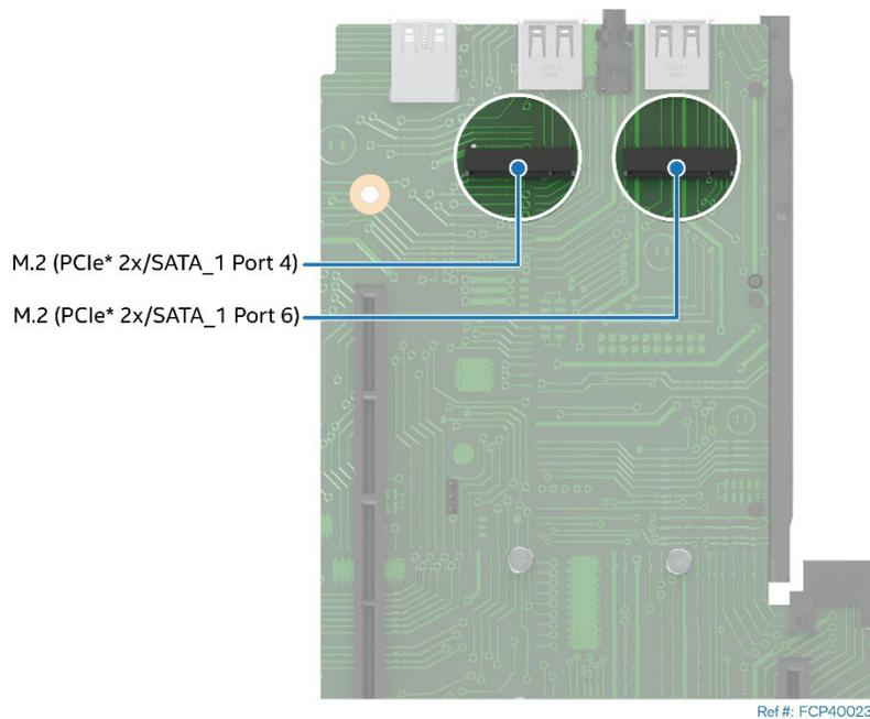
**Figure 89. M.2 Module Connector Location**
