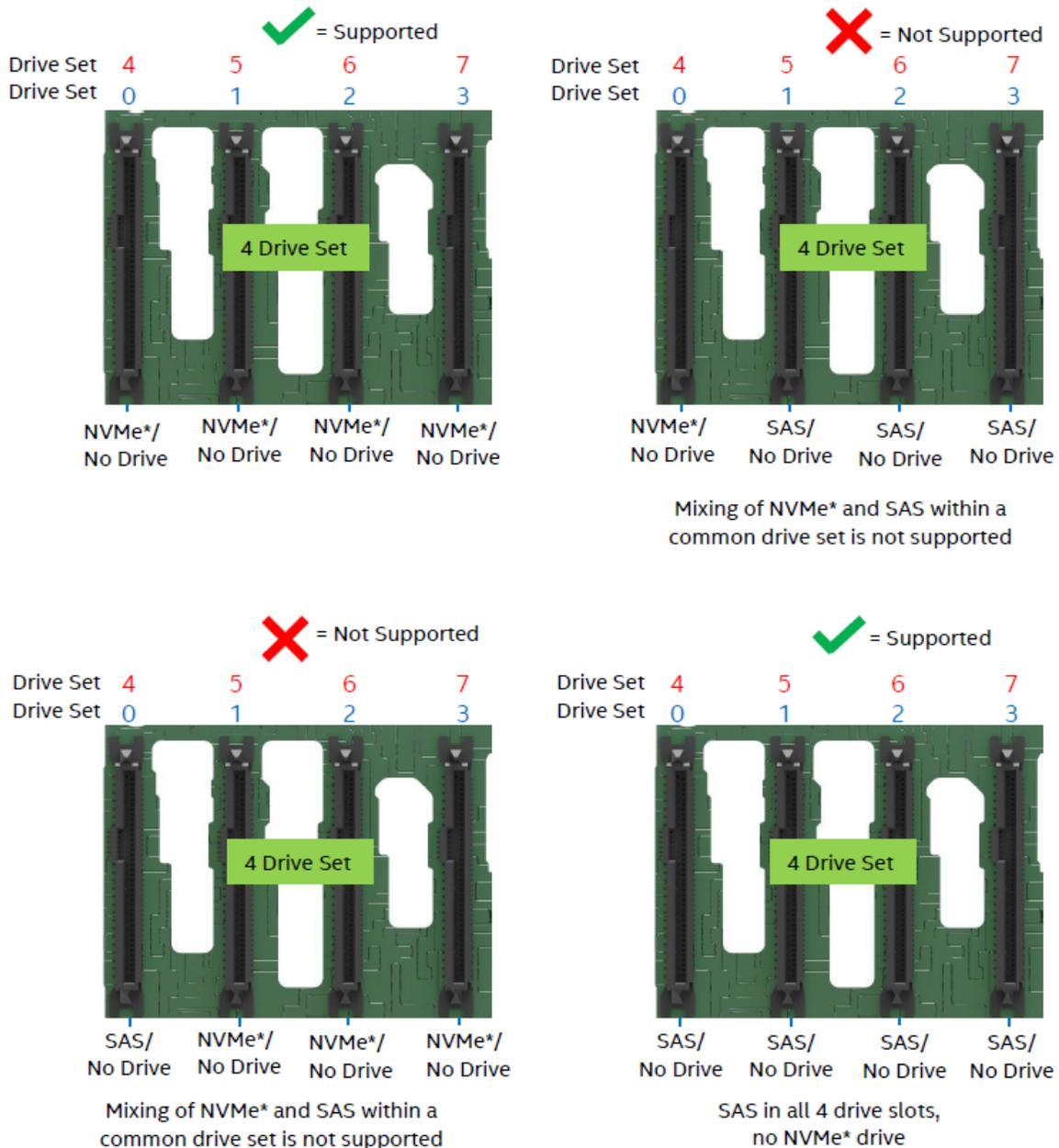
**Figure 85. Supported Drive Population for Server Board MCIO Connectors or Tri-Mode Intel® RAID Module**
