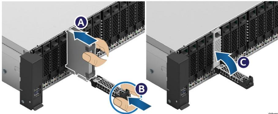
Figure 60. 7-mm Drive Insertion into 2.5" Drive Bay
