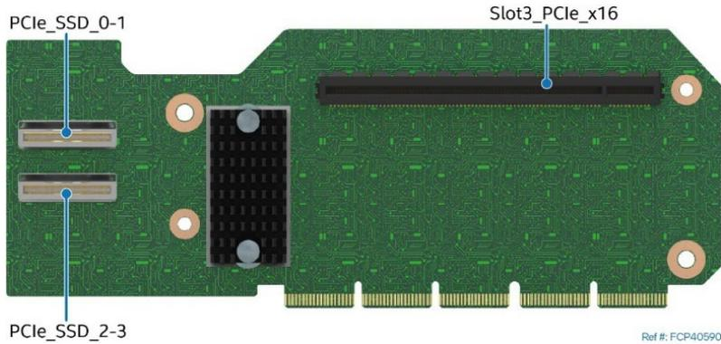
Figure 82. PCIe\* NVMe\* Riser Card for Riser Slot #1
