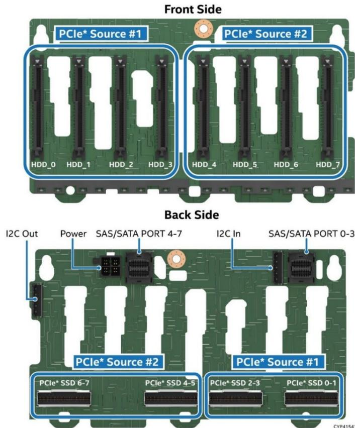
Figure 84. Backplane Cabling from Two Backplane Sources
