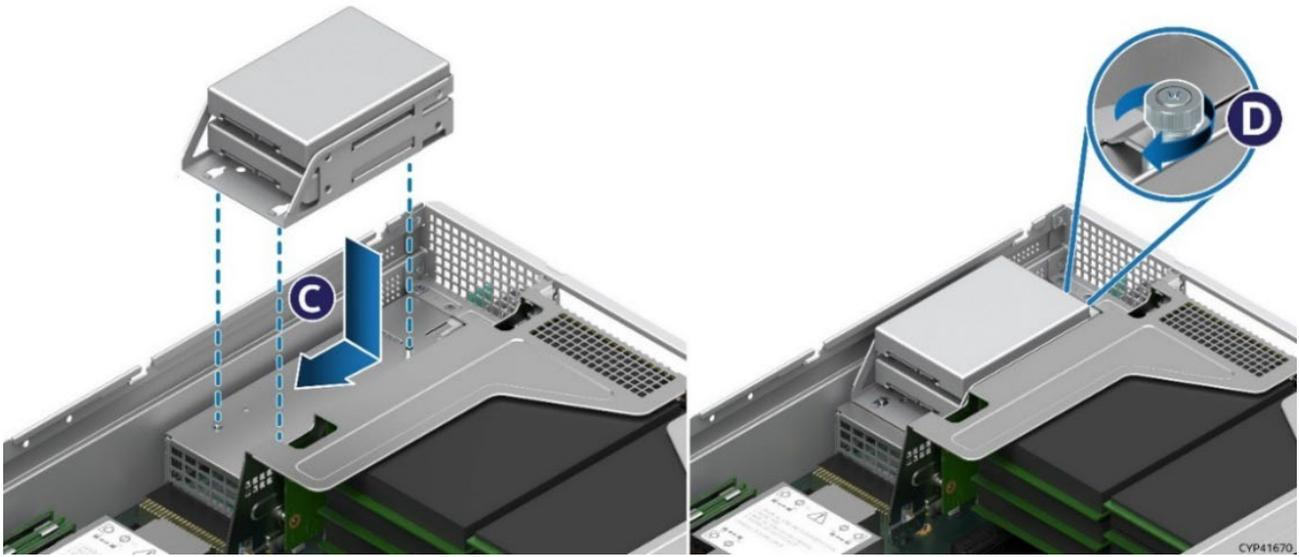
**Figure 90. 2.5" Solid State Drive (SSD) Mounting Option**
