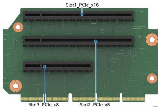
**Figure 50. Three-slot PCIe\* Riser Card for Riser Slot #2**
