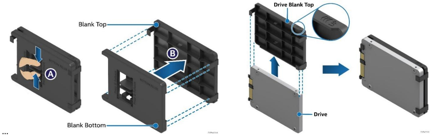
Drive installation into the front drive bay and extraction from the front drive bay is the same for both 7mm and 15mm height drives.
