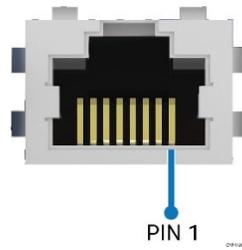
**Figure 98. RJ45 Serial Port A Connector Pin Orientation**
