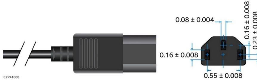
**Figure 32. AC Power Cord Specification**
