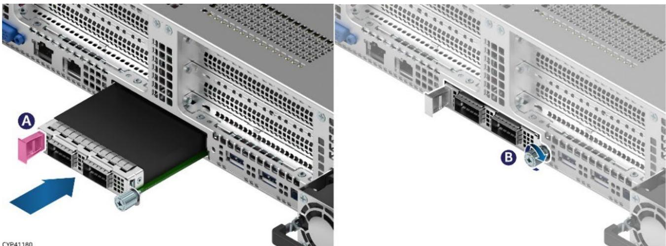
**Figure 58. OCP\* Adapter with Pull Tab Installation**
