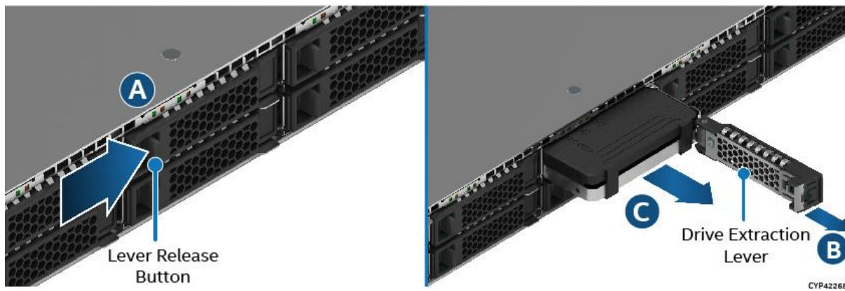
Figure 63. 7 mm Drive Removal from 2.5" Drive Bay
