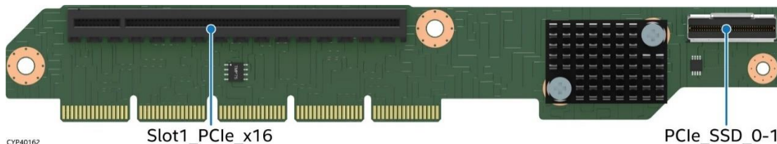
Figure 50. PCIe* NVMe* Riser Card for Riser Slot #2
