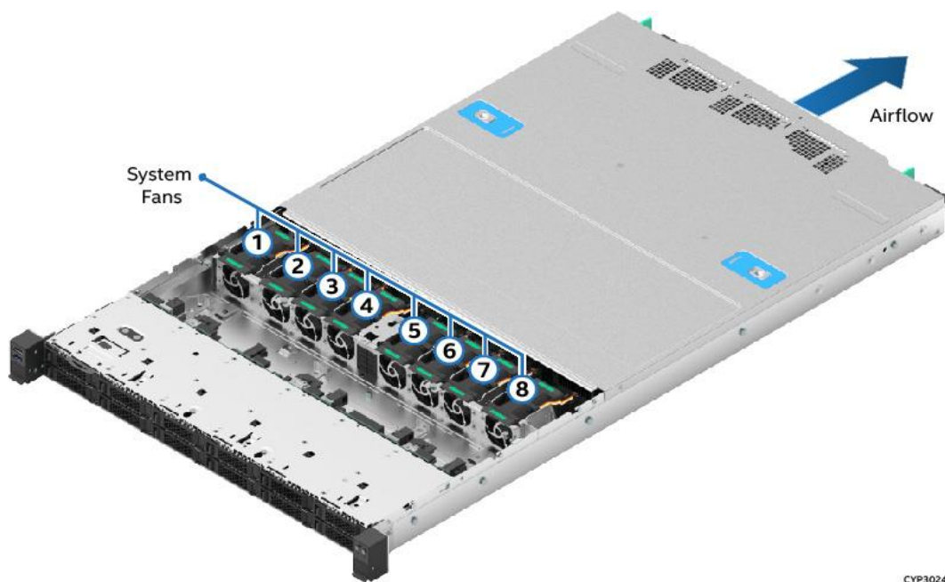
Figure 35. System Airflow and Fan Identification
