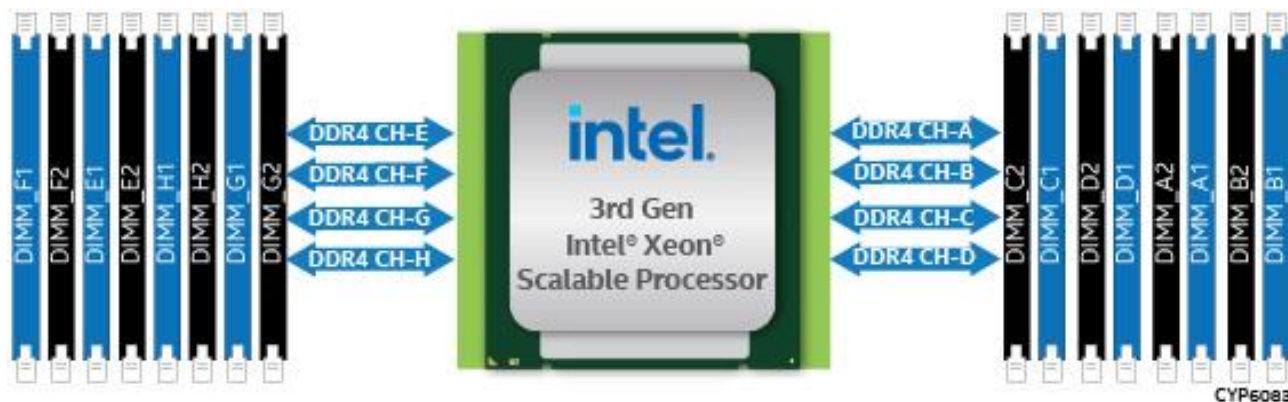
Figure 23. Memory Slot Connectivity
