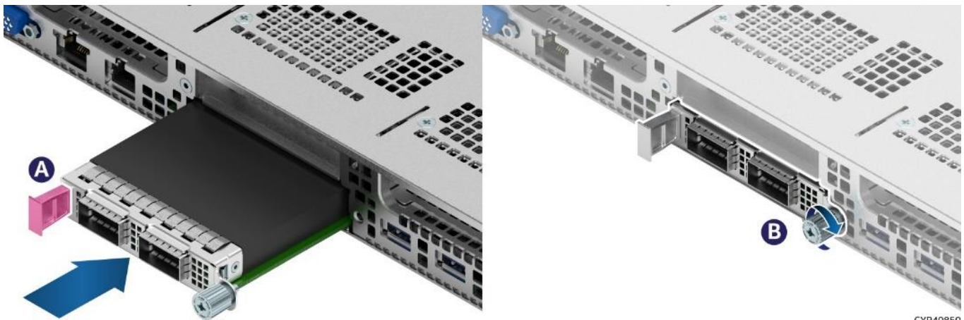
Figure 55. OCP* Adapter with Pull Tab Installation
