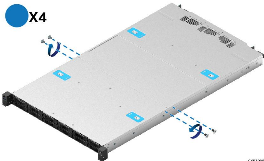
Figure 16. System Top Cover Shipping Screws
