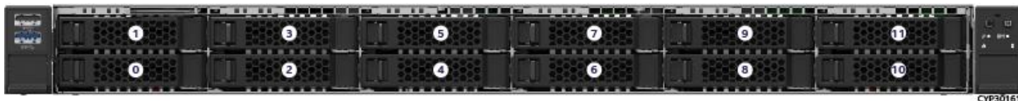
Figure 57. 12 x 2.5" Front Drive Bay Configuration – M50CYP1UR212
