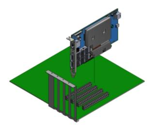
3. Hold the card by its edges and bracket, avoiding contact with the top surface. Apply even pressure to both edges of the card and gently insert the BlueField-3 card into the PCI Express slot.
