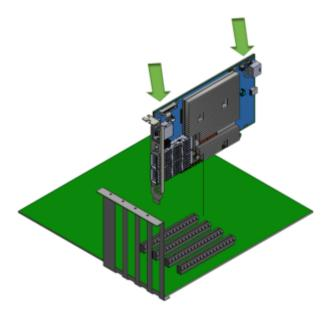
4. When the BlueField-3 card is properly seated, the port connectors are aligned with the slot opening, and the card's faceplate is visible against the system chassis.
