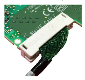
**Step 5:** Slide the Cabline CA-II Plus harnesses through the retention clip. Make sure that the clip opening is facing the plugs.
