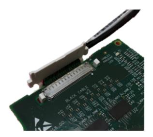
Step 9: Clamp the retention clip. Verify both latches are firmly locked.
