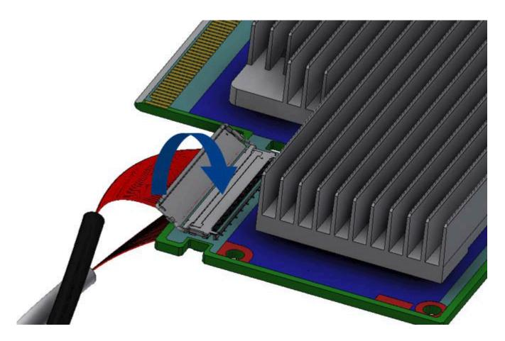
**Step 4:** Slide the retention clip latches through the cutouts on the PCB. The latches should face the annotation on the PCB.
