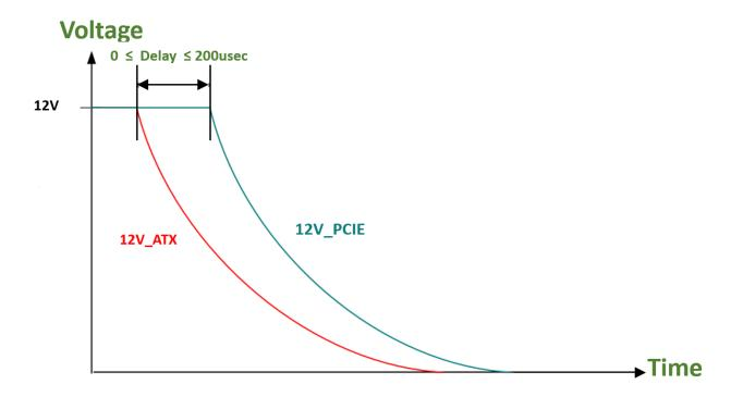
2. The 12V\_PCIE voltage must not be powered down while the 12V\_ATX voltage is powered up.
