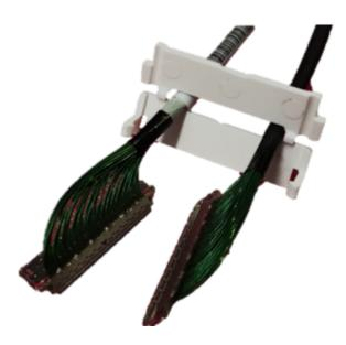
**Step 6:** Plug the Cabline CA-II Plus harnesses on the PCIe Auxiliary Card. As indicated on both sides of the Auxiliary connection card; plug the black harness to the component side and the white harness to the print side.
