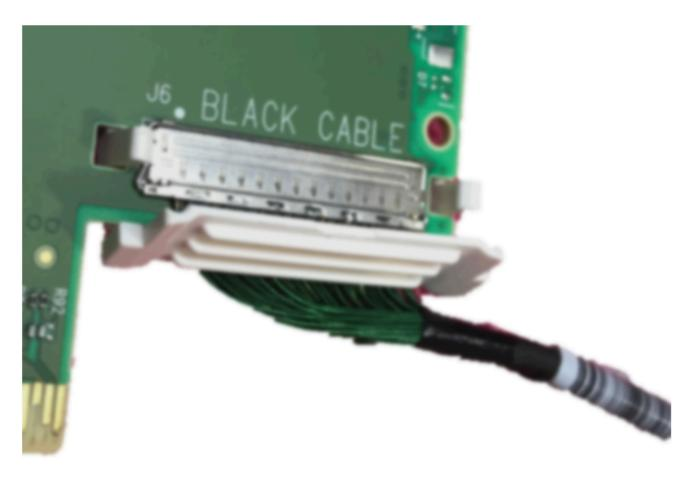
**Step 4:** Clamp the retention clip. Verify both latches are firmly locked.
