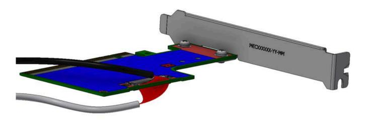
**Step 8:** Slide the retention clip through the cutouts on the PCB. Make sure latches are facing "Black Cable" annotation as seen in the below picture.
