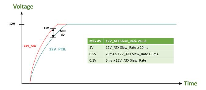
2. The 12V\_ATX can be powered up after the 12V\_PCIE, with a maximum delay of 2 seconds. The below graph illustrates the delay between the 12V\_ATX and 12V\_PCIE voltages at power-up.
