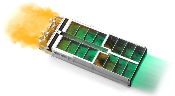
Figure 2. Ultrastar Data102 showing thermal zones and airflow
